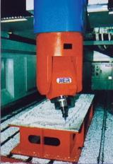
Dual-swiveling milling head of electric spindle driven by torque motor
