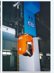
Dual-swiveling milling head of mechanically driven electric spindle
